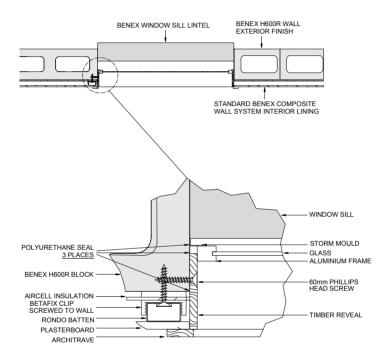
Fixing Windows to Benex is faster than other wall systems as frames are directly screw fixed into the Benex Opening with standard & appropriate Class 3 External Grade screws. No "Wall Plugs" required.
